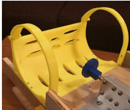
FIGURE 3: 3D PRINTED BAG HOLDER
