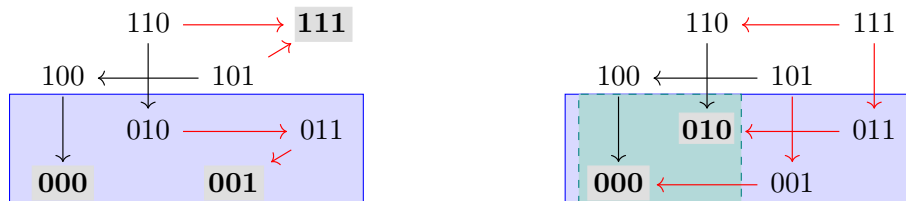
Figure 3.4: Asynchronous dynamics of the Boolean function f(x) = (x_1x_3, x_1x_3 \vee x_2\bar{x}_3, \bar{x}_1x_3 \vee x_2) (left) and f^C(x) = (0, x_2, 0) with \mathcal{C} = \{(3, 0)\} (right). Transitions that vary between AD(f) and AD(f^C) are marked in red. Attractors are marked in bold and gray background. T = 0*0* (blue) is a trap space only containing attractors belonging to P = 00* . \mathcal{C} is a transient control strategy for P since \mathbb{B}^n percolates to T' = 0*0 (green) under f^C , with T' \subseteq T . \mathcal{C} is not a permanent control strategy for P since AD(f^C) has a steady state (010) not contained in P .
