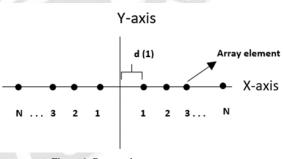
Figure 1. Proposed antenna array geometry
