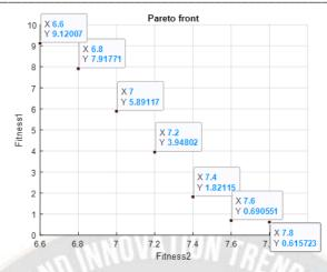
Figure 2. Pareto front obtained for the hybrid Chebyshev based MO-GA
