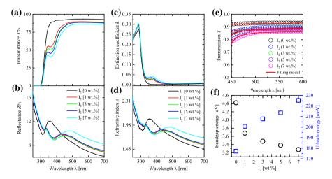
**Fig. 6** a Transmittance, **b** reflectance, **c** extinction coefficient, and **d** refractive index spectra of PEO: $I_2$  films for different  $I_2$  concentrations, **e** Transmittance spectra of PEO:  $I_2$  films for different  $I_2$  concentrations; experimental (colored circles) and model calculated (solid red lines). **f** Band-gap energy ( $E_g$ ) and Urbach energy of PEO: $I_2$  films as a function of  $I_2$  concentrations (colour figure online)
