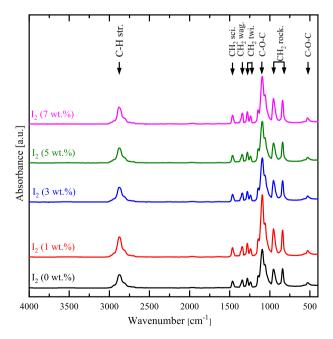
Fig. 1 FTIR spectra of pure PEO and PEO:I<sub>2</sub> complex composites with varying I<sub>2</sub> doping concentrations
