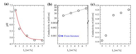
Fig. 3 a pH and b electrical conductivity of PEO:I<sub>2</sub> composite solutions versus I<sub>2</sub> [wt%], and c Electrical conductivity of PEO:I<sub>2</sub> composite films versus I<sub>2</sub> [wt%]
