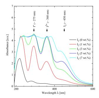
Fig. 4 Absorbance spectra for PEO: I<sub>2</sub> composite solutions
