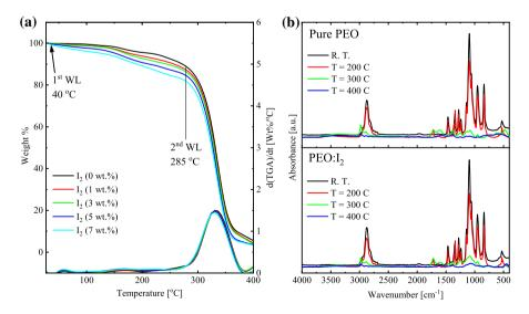
**Fig. 5** a TGA and d(TGA) curves for PEO:I<sub>2</sub> composite films for varying I<sub>2</sub> concentration, **b** FTIR spectra of pure PEO and PEO:I<sub>2</sub> (5 wt%) films for varying annealing temperatures
