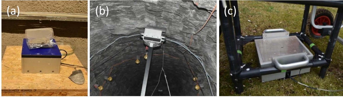
Figure 1. Potential application fields for single-sided (SiS) NMR in geosciences: (a) mobile NMR for investigating samples immediately after taking them, i.e. an analysis without the risk of chemical altering or evaporation, (b) in-situ moisture measurements on tunnel walls, e.g. a relevant contribution to the stability and integrity assessment of underground facilities, (c) non-invasive soil moisture measurements.
