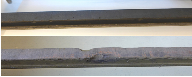
Figure 1. Top: used collector strip with clear abrasion marks on the edges. Bottom: used collector strip with serious damage.
