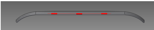
Figure 4. Collector strip with schematic representation of integrated fibre optical sensors (red). They are positioned on the boundary between the aluminium profile and the carbon bar, close to the edge, and were used successfully to detect hits in a horizontal (driving) direction.
