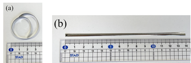
FIG. 3. Photographs of the long Fe-Ni bilayer ribbons before and after the joule-annealing. (a) As-peeled ribbon (b) Joule-annealed ribbon.
