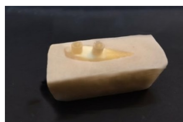
Figure 5: Samples prepared for the shear bond strength test
