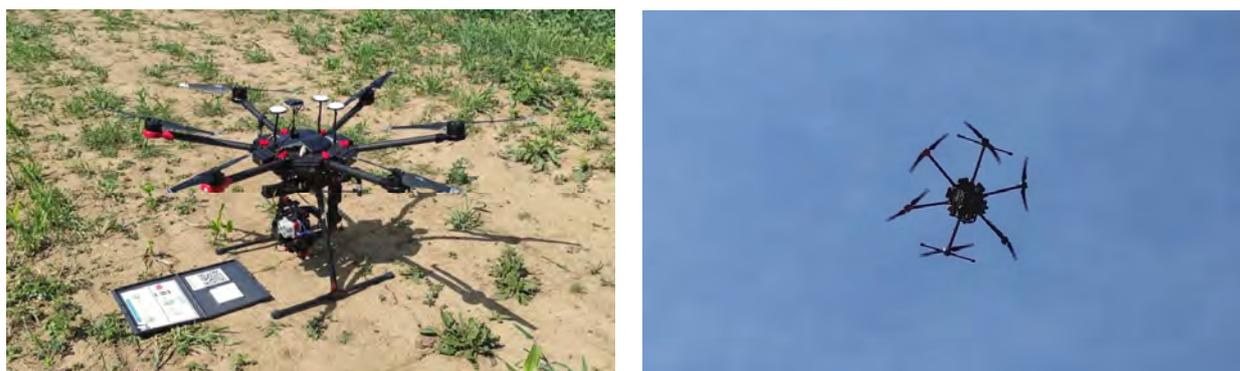
**Figure 3.** The six-rotor UAV DJI Matrice M600 with Micasense Altum camera on the ground with calibration panel (left) and during the flight (right).
