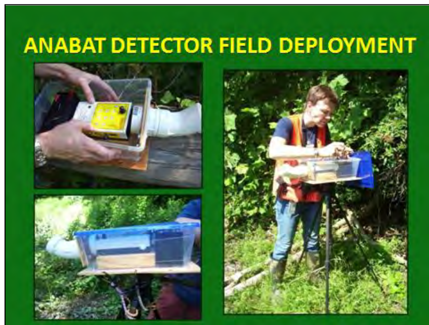
Figure 8: Anabat SD-2 Field Deployment in Weatherproof Housing
