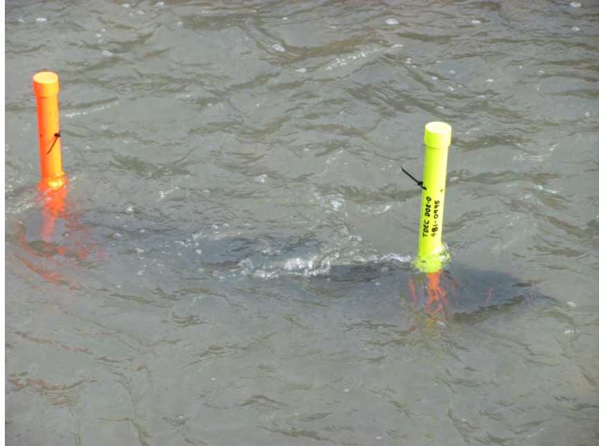
Figure 2.1.6.2.4 Sediment trap deployed
