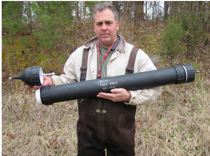
Figure 2.1.6.2.3 Photo of sediment trap
