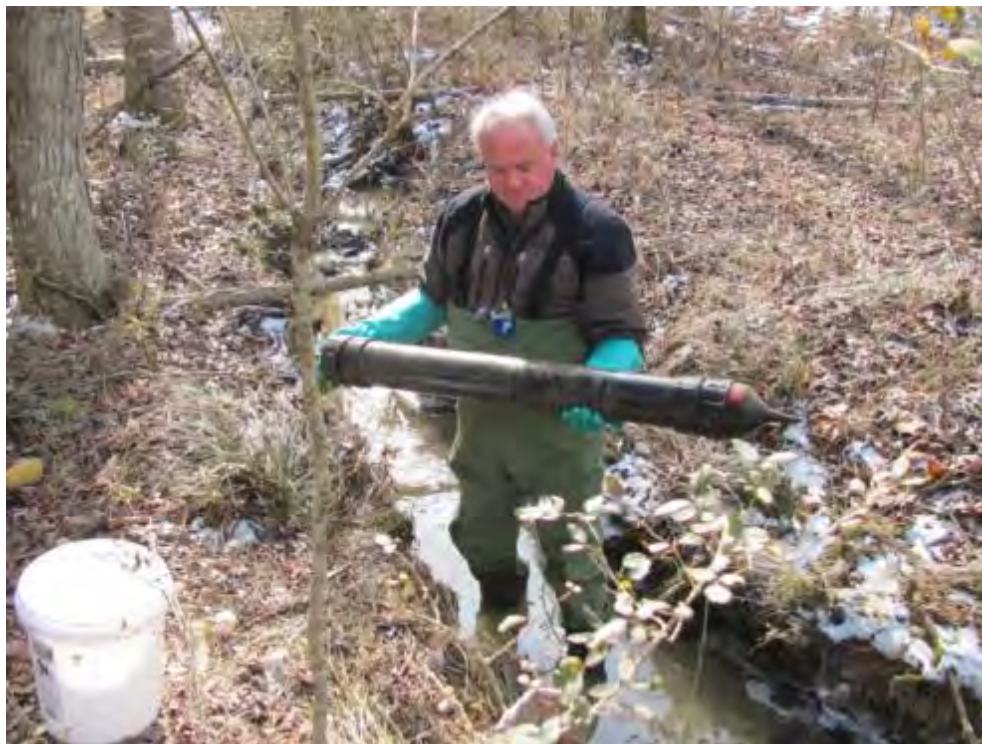
Figure 2.5.2.3: Photo of Sediment Trap
