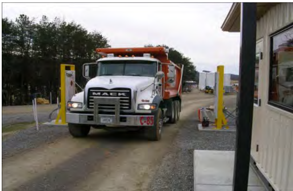
Figure 2.1.3: Truck Hauling Waste through the Portal Monitor
