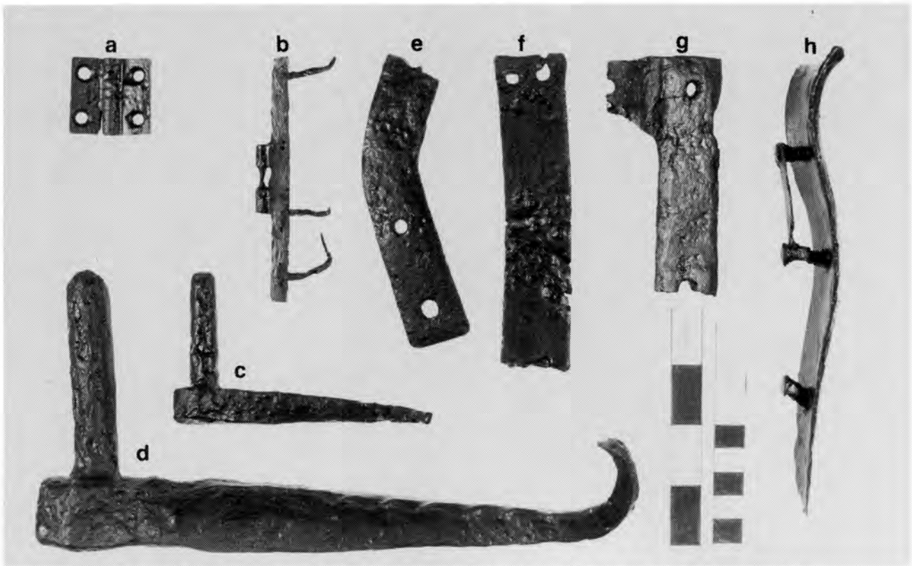
Figure 47. Construction hardware: (a) butt hinge; (b) H hinge; (c) door or shutter pintle; (d) gate pintle; (e) angle brace; (f) strap brace; (g) corner bracket; (h) saddle brace or hinge fragment.
