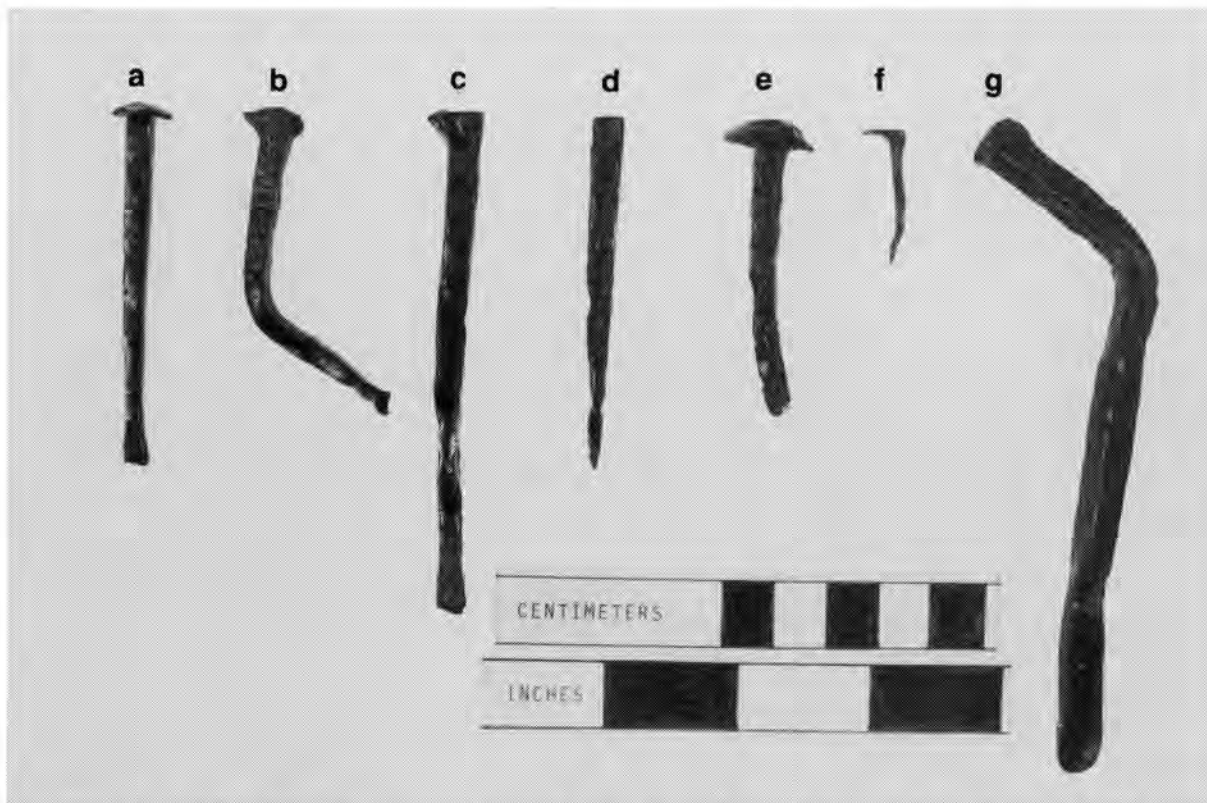
Figure 46. Hand-wrought nails and spikes: (a) rosehead nail with spatulate point, (b) T-head nail with spatulate point, (c) L-head nail with spatulate point, (d) headless nail with sharp point, (e) mushroom head nail with spatulate point, (f) tack, (g) L-head spike.
