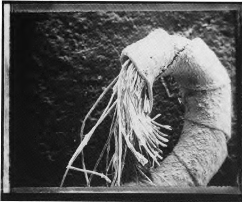
Figure 81. Weft yarn of metallic ribbon (84-90-53-5) showing silk core with silver foil wrapping. Photograph taken at 100X.
