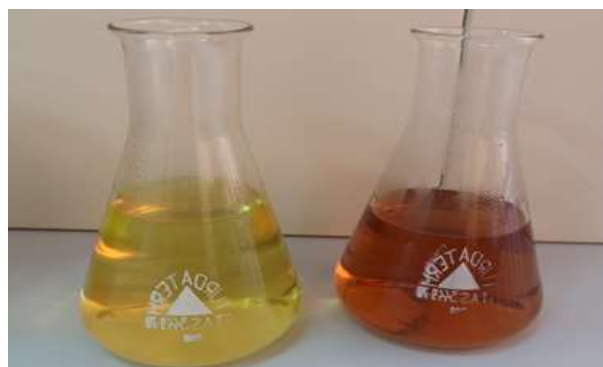
Figure 1 Color shifting from yellow to reddish brown indicating the formation of green silver nanoparticles
