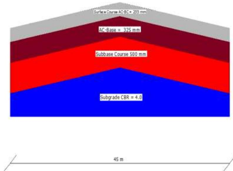
**Gambar 7.** Tebal Lapisan Eksisting Perkerasan STA 0+000 – 1+800
