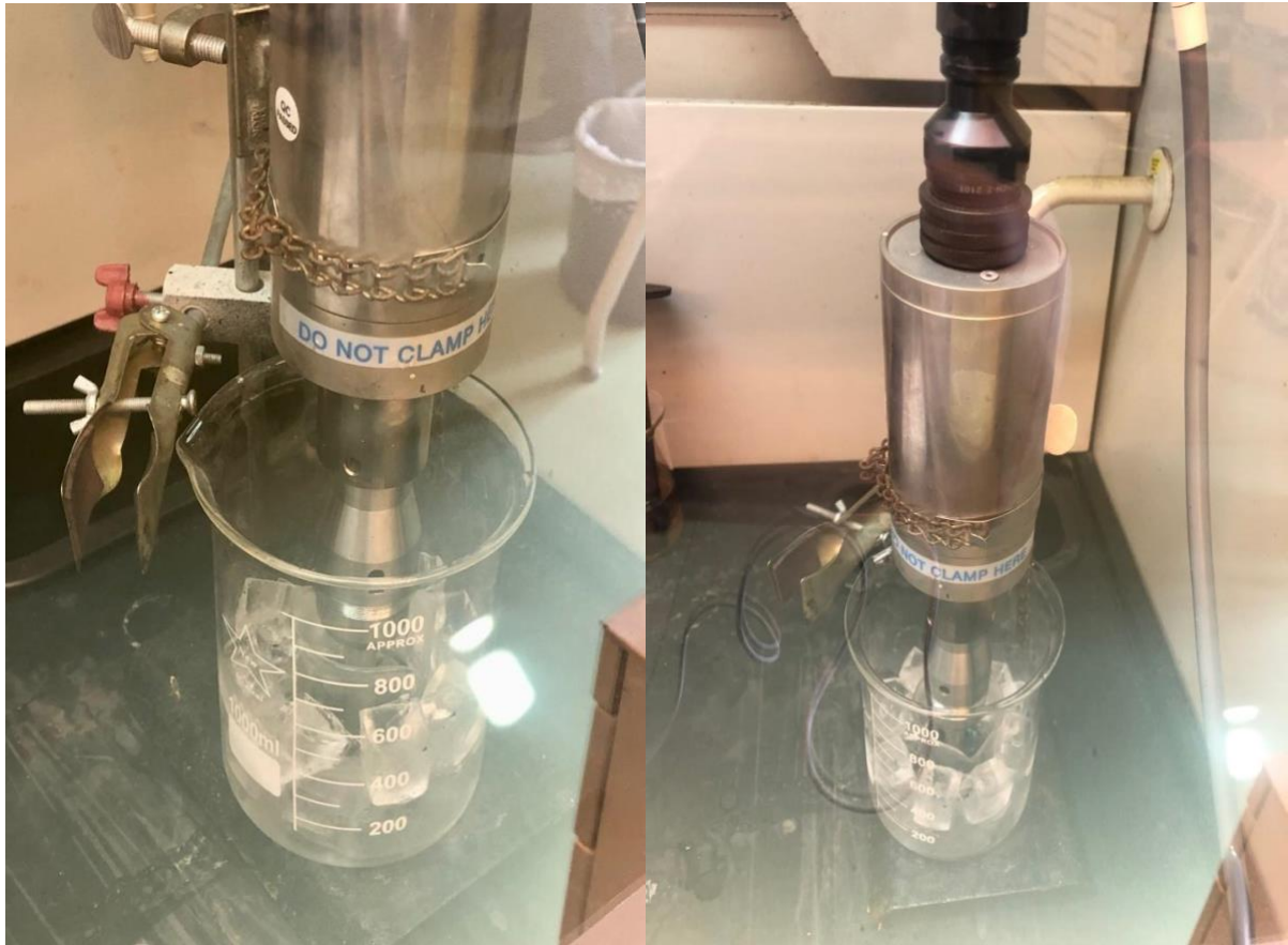
Figure 8 Sonication of MWCNTs in DMF within an ice bath
