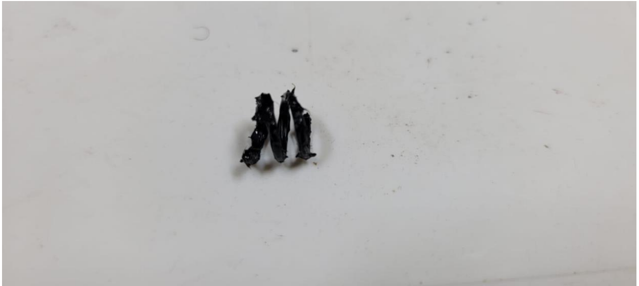
Figure 9 Fully functional Spring Sensor after coating and thermal treatment
