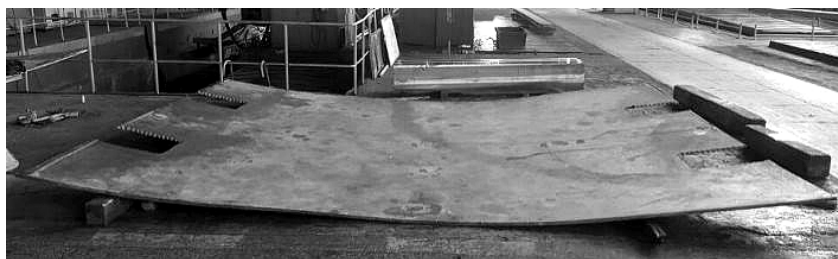
Fig. 1. Deformation of stainless clad plate after heat treatment.
