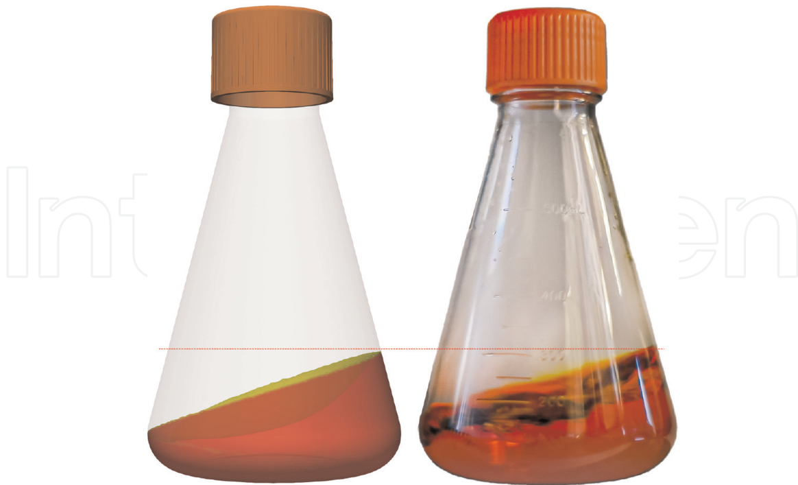
Figure 9. Simulation (left) and experiment (right) of the fluid flow in a 500 mL shake flask with 150 mL of working volume at 160 rpm and 25 mm shaking amplitude. The dashed red line indicates the empirically calculated maximum fluid height according to Büchs et al. [33], which deviates by only 2% from the simulated one.
