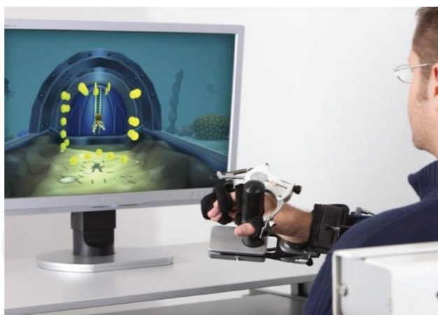
Figure 5. Integrated neuroprosthesis with a gravity-compensating, seven degree-of-freedom exoskeleton, Armeo Spring exoskeleton, Hocoma, and virtual environment feedback attached to the paretic arm [50].
