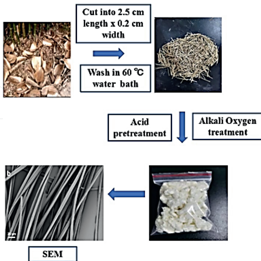
Figure 3. Degumming process of BSSF [29].
