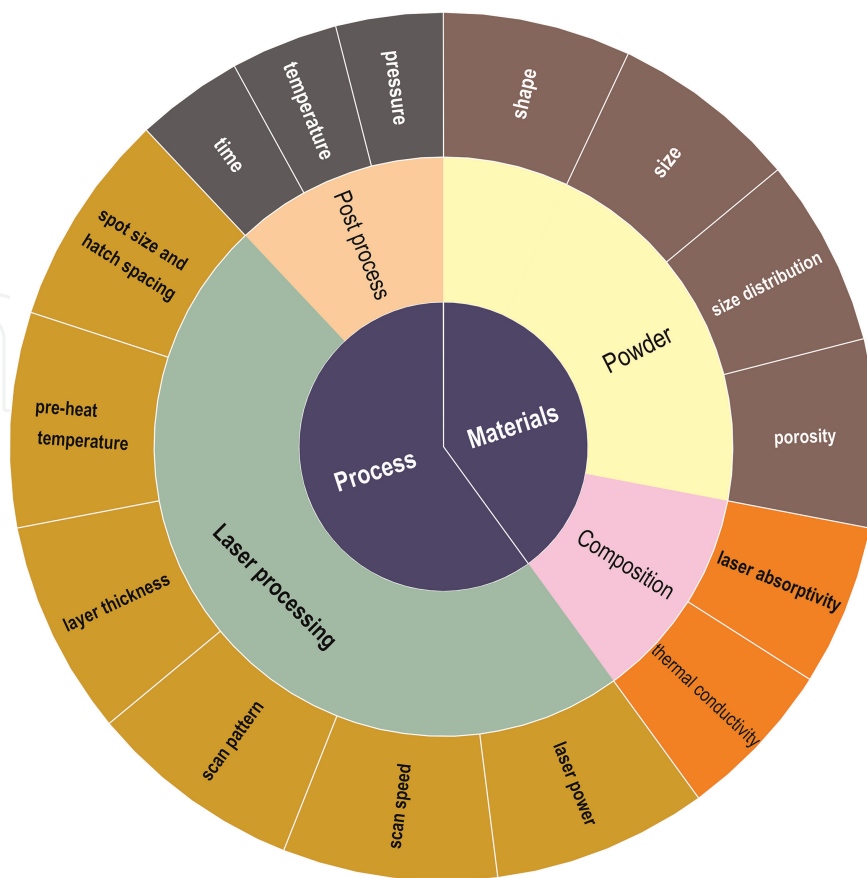
Figure 3. Factors influencing the properties in additively manufactured HSAAs.
