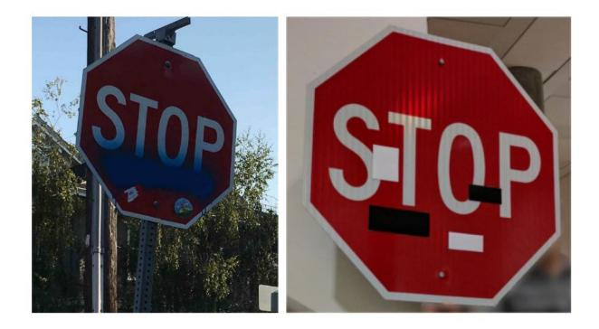
Figure 4: Stop sign classified as speed limit sign
