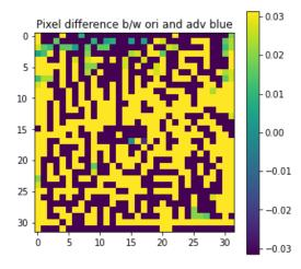
Figure 26: pixel difference b/w original and adversarial for the blue channel
