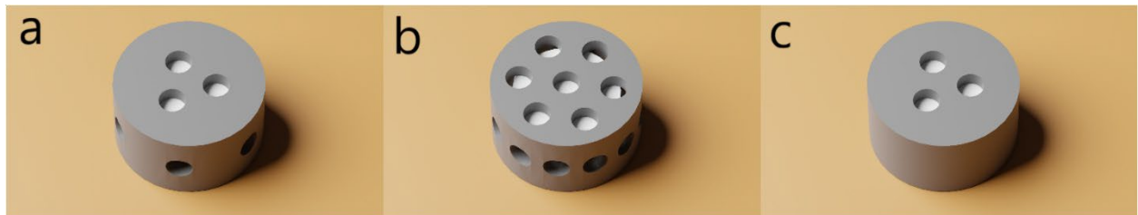
Fig. 2. The different types of tablet design. a) Three holes on the top and bottom with six holes on the side. b) Seven holes on the top and bottom with twelve holes on the side. c) Only three holes on the top and bottom.
