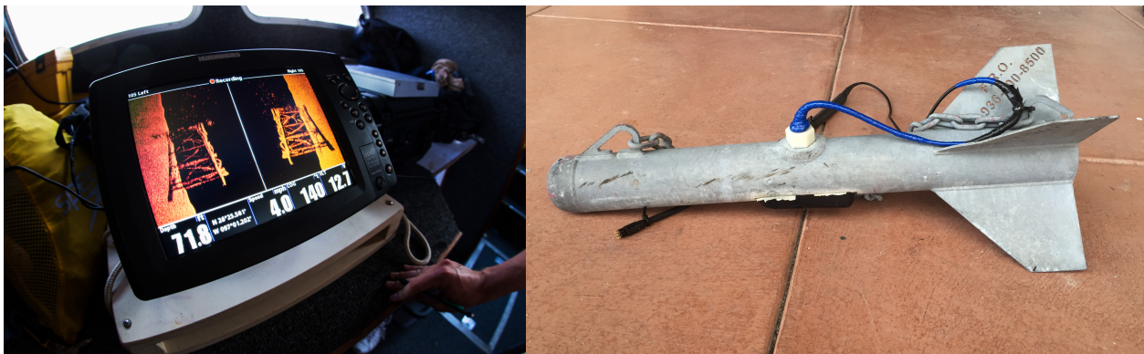
Figure 2. Humminbird 1198c head unit and towfish used in this study
