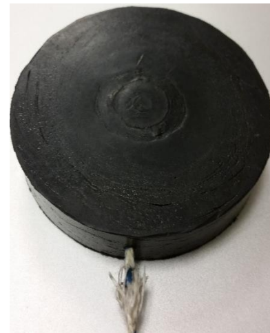
Figure 2. Hysteresis heating cylindrical specimen with thermocouple.
