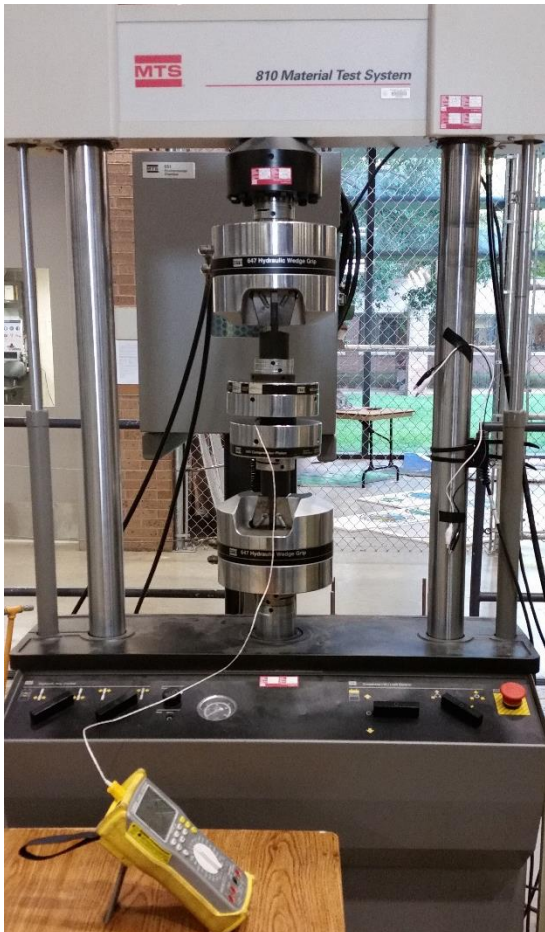
Figure 3. Hysteresis heating test setup on MTS 810 Material Test System [5].
