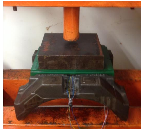
Figure 11: Class K Bearing Adapter Test with Pad-Liner: 4-Leg Support and Top Applied Pressure
