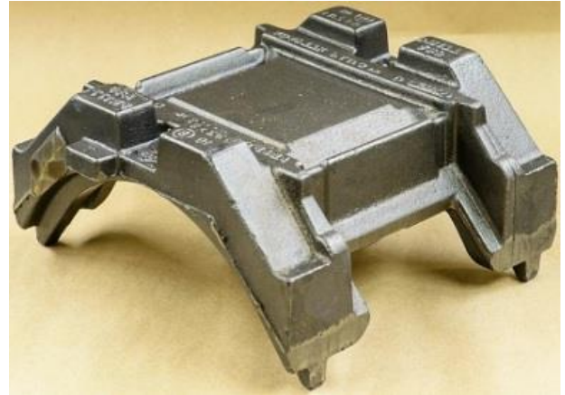
Figure 2: Original Railroad Bearing AdapterPlus™ without Elastomer Pad-Liner
