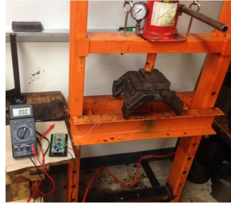
Figure 10: Class K Bearing Adapter Test without Pad-Liner: 4-Leg Support and Top Applied Pressure
