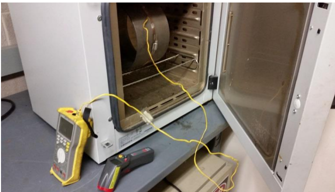
Figure 9. Oven test setup. The K-type thermocouple can be seen attached using a hose clamp. The thermocouple multi-meter can be seen attached at the other end of the thermocouple.
