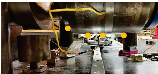
Figure 5. Infrared scanning locations from left to right: inboard seal, inboard raceway, spacer, and outboard raceway
