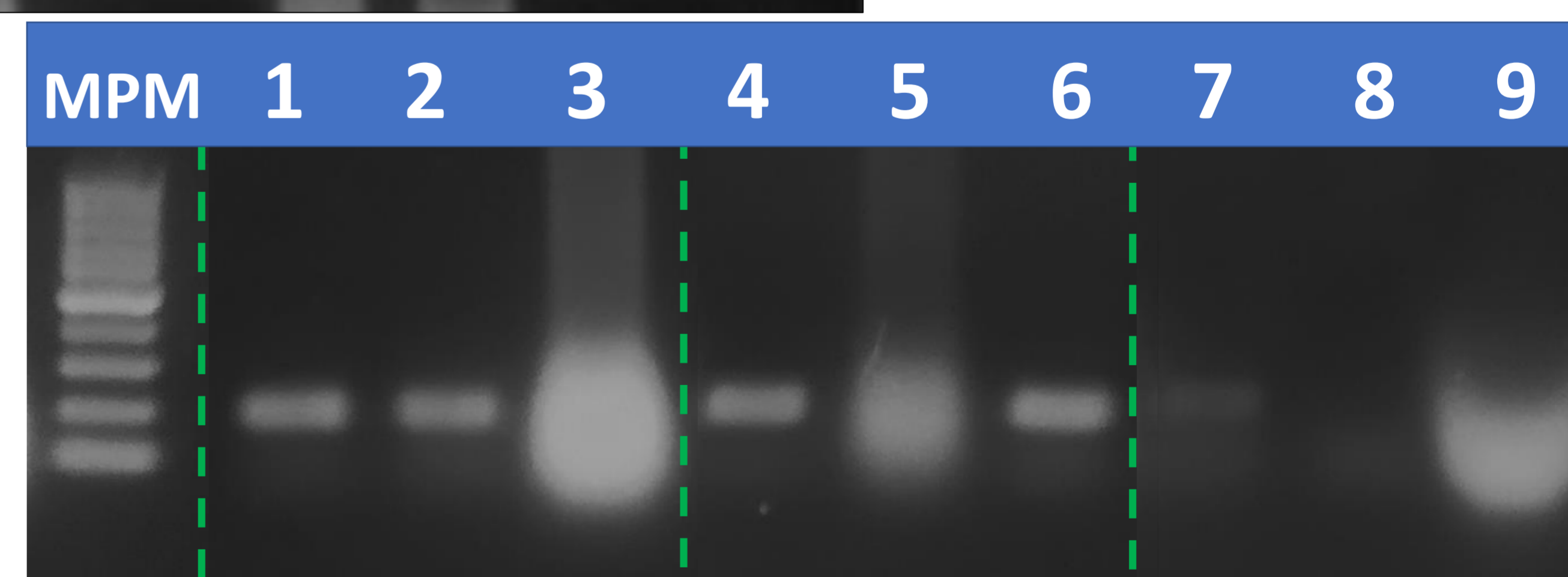
Figure 2. 1% Agarose gel. Amplifications of Alfalfa DNA samples of hay, seeds and fresh leaf. DNA extractions by Commercial Kit method (rows 1, 4 & 7), SDS method (rows 2, 5 & 8), and Potassium Acetate method (rows 3, 6 & 9).
