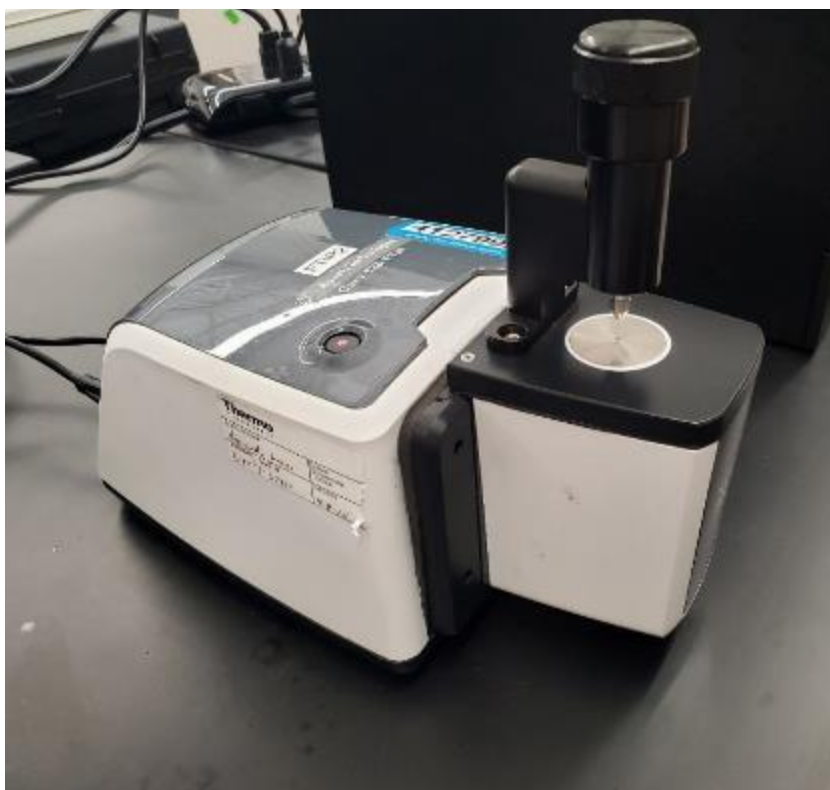
Figure 22: Cary FTIR with ATR attachment
