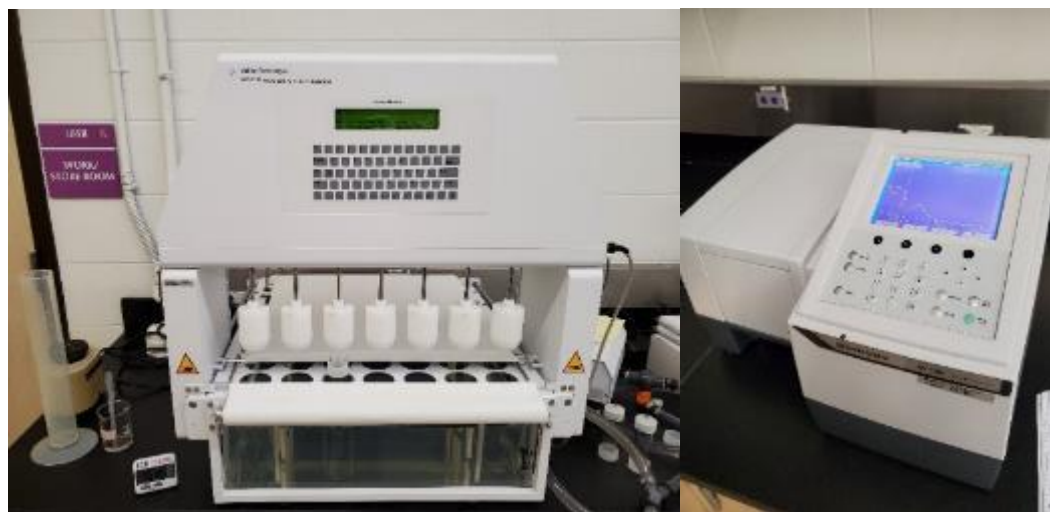
Figure 18: BIO-DIS Reciprocation Cylinder Apparatus (Left), UV-1280 Multipurpose UV-Visible Spectrophotometer (Right)
