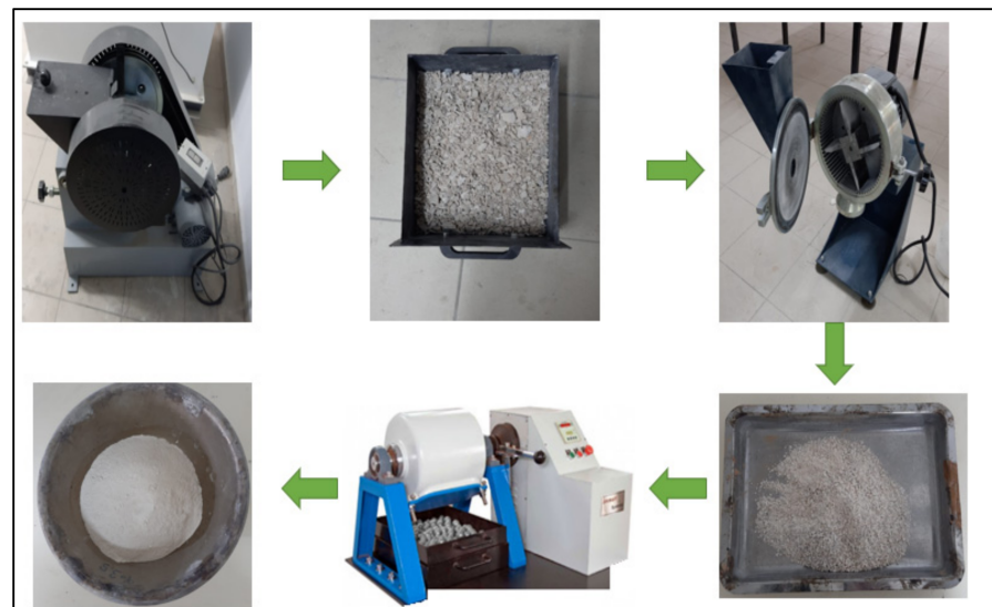
Figure 1. Production stages of firebrick powder.
