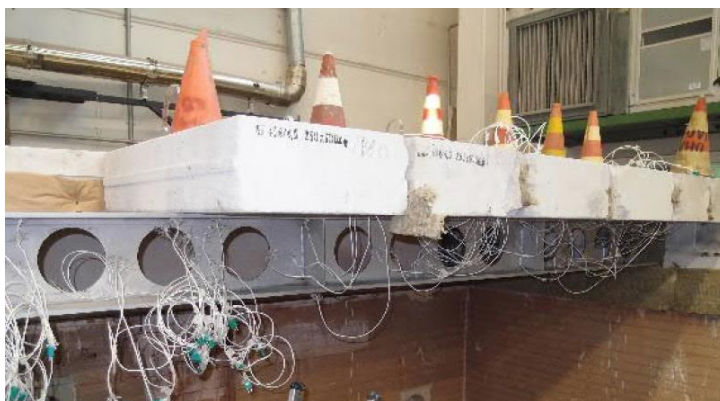
Figure 1 Cellular beam prior to fire testing [7].
