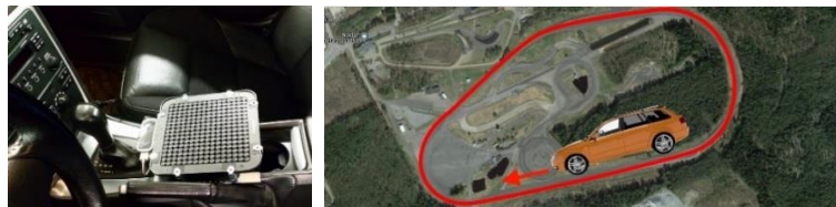
Figure 4. Car setup: Ultrahaptics device location (left) and test track layout (right).
