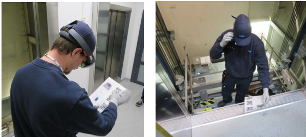
Figure 2. User scanning the QR-code to start the instruction (HoloLens on the left, and Vuzix on the right).
