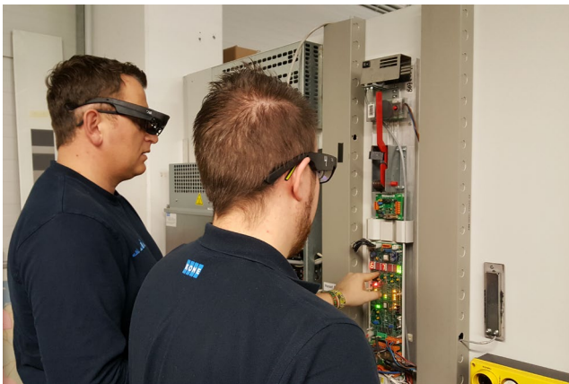
Figure 8. A maintenance expert is performing maintenance task using ODG R-7. Another one is following the work and instructions on ODG R-7.
