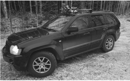
Fig. 1. Recording platform. Our vehicle is equipped with four Basler HD cameras, a NovAtel GNSS antenna, and a KVH 1750 IMU with fiber optic gyro.
