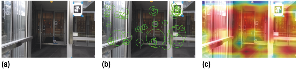
Figure 2.3 Extraction of feature information from a sample images using (a) ArUco Marker detected in the scene (b) ORB features detected in the image (c) Activation map of the deep features, extracted using VGG-16 network, overlaid over the sample image.
