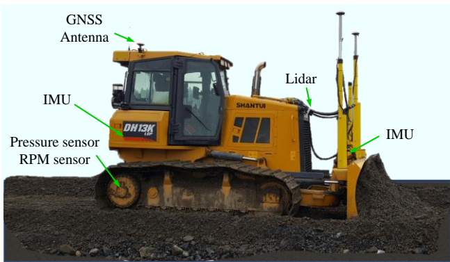
Fig. 4. The experimental setup and sensors installed on the machine. Masts on the blade are not used in this study.
