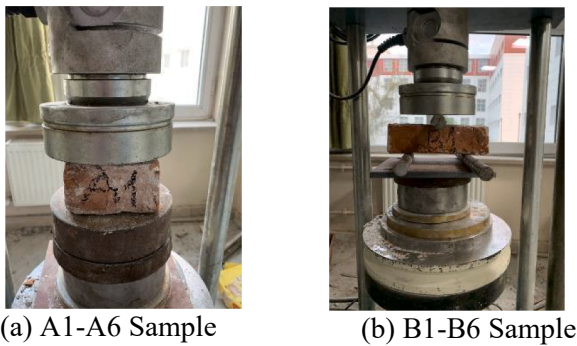
Fig. 2. a) Compressive strength test of brick, b) Flexural tensile strength of the bricks.
