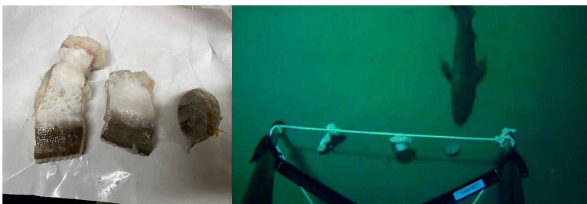
Figure 4. Acoustic tags wrapped in fish fillet and king prawn (left) and attached to the tripod for exposure to the cod. Image from the underwater video camera (right) shows the moment when the king prawn was eaten by an approaching cod.
