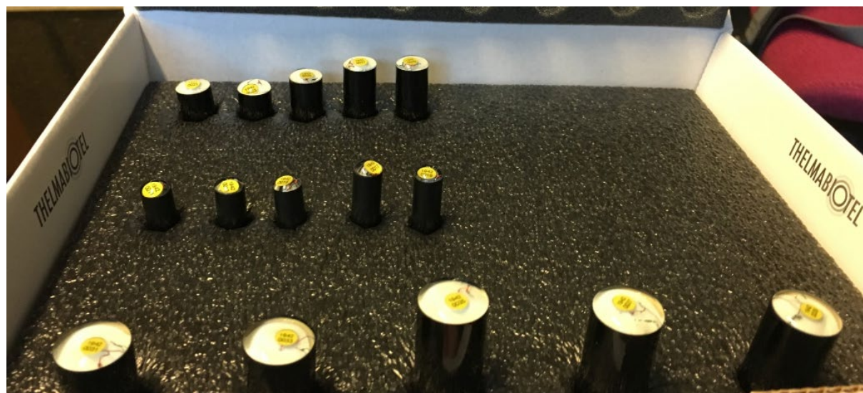
Figure 1. The three sizes of acoustic tags that were provided by Thelma Biotel. 13 mm \varnothing top row, 9 mm \varnothing middle row, 16 mm \varnothing bottom row.
