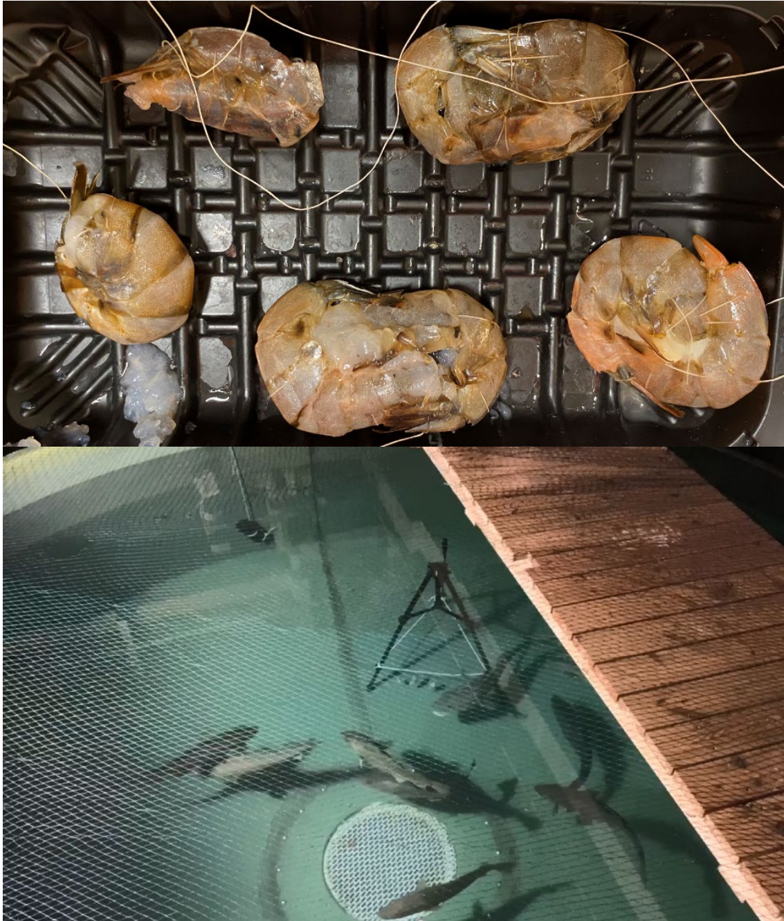
Figure 5. Acoustic tags baited with king prawns and sewn together with cotton (top image). Small tags ( \varnothing 9mm) were able to fit into one prawn, while 2 prawns were used to better encapsulate the medium and large tags ( \varnothing 13 and 16 mm). Baited acoustic tags hanging from the tripod in the large seawater tank, receiver positioned on the wall of the tank.
