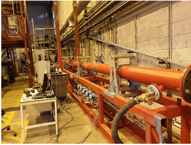
Fig. 1 Picture of the flow loop test section in a horizontal position
