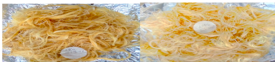
(e) 5% NaOH treated Sisal ( S_{5\%} ) fiber
