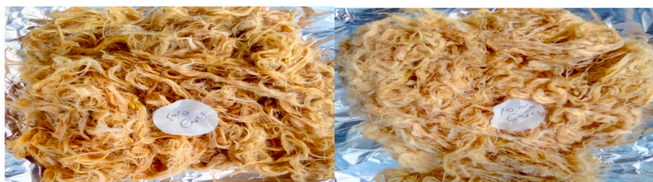
(c) 5% NaOH treated Enset ( E_{5\%} ) fiber
