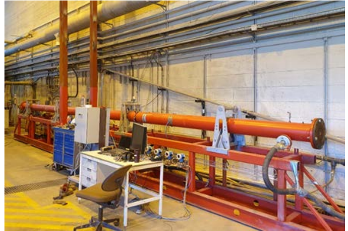
FIGURE 1. PHOTO OF THE FLOW LOOP TEST SECTION IN HORIZONTAL POSITION.
