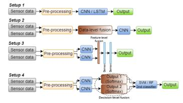
Fig. 2: Experimental setups for different model configurations. Setup 1: single sensor data model; Setup 2: data-level fusion; Setup 3: feature-level fusion; Setup 4: decision-level fusion.
