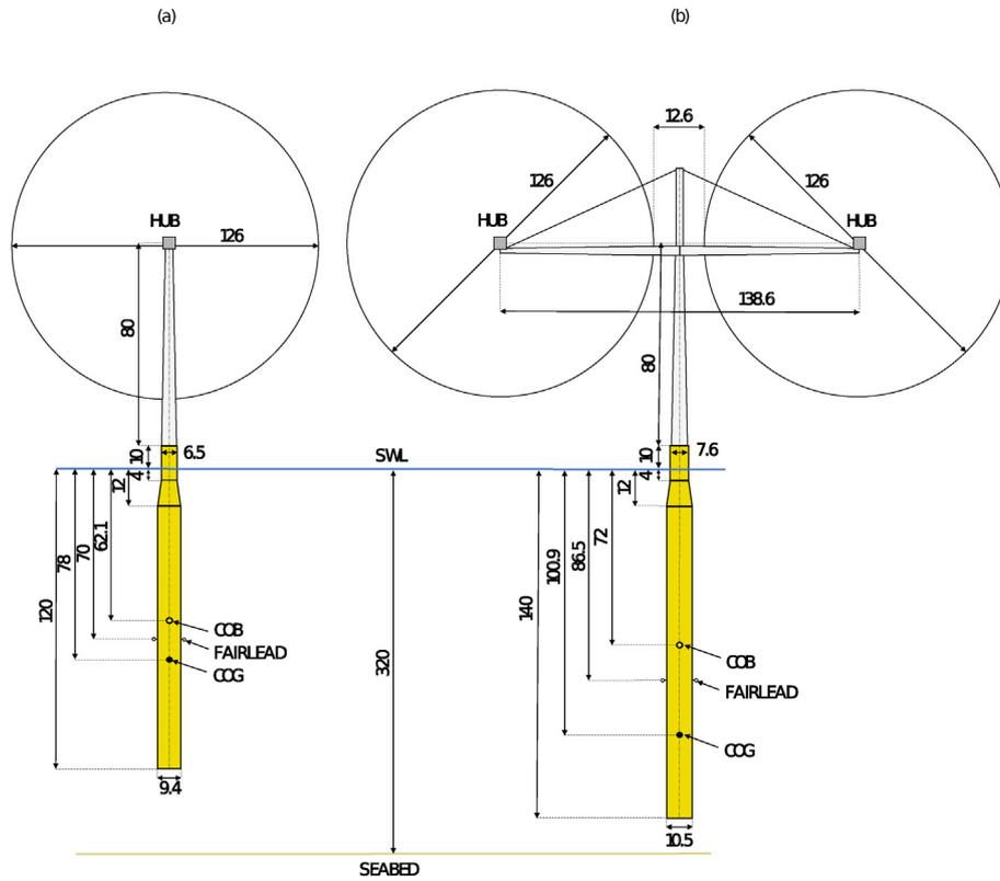
Fig. 2. a) OC3 geometry [m] [14]. b) 2WT configuration [m] [13].
