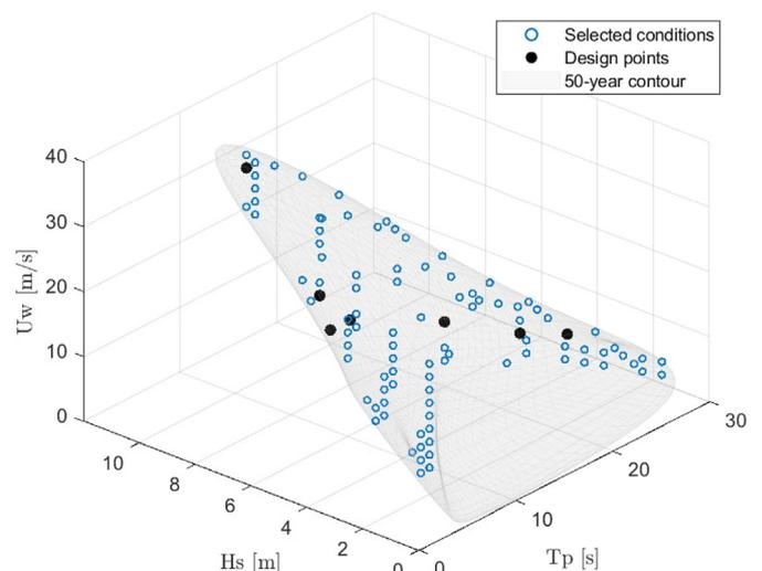
Fig. 8. Discretized conditions for 50-years contour surface for site 3. The blue circles are the selected conditions, while the filled black circles are the design points.
