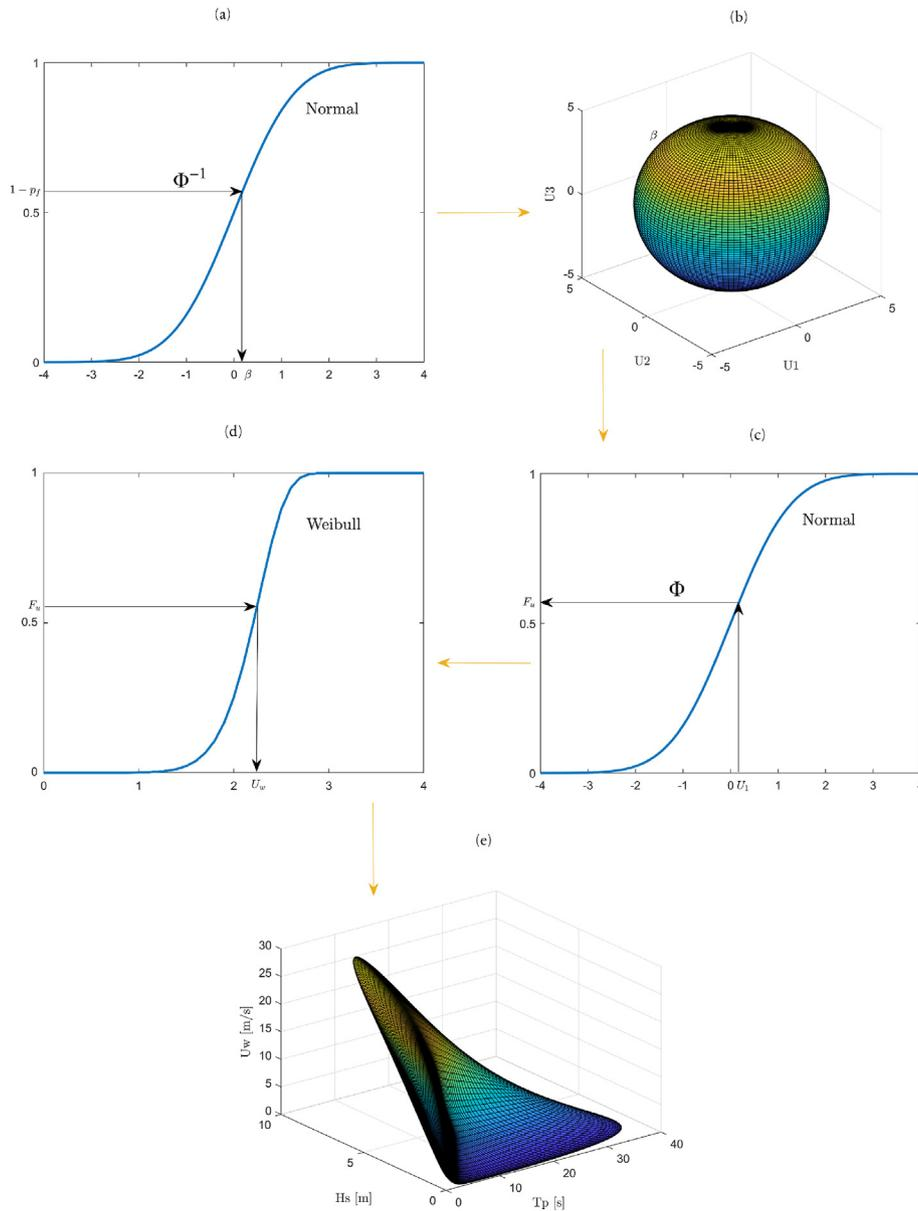
Fig. 1. Graphical representation of the Environmental Contour Method (ECM), based on Roseblatt transformation [12]. Only the marginal (Weibull) distribution of  $U_w$  is shown, relative to a standard height of 10 m and site 14 (Table 3) [7].
