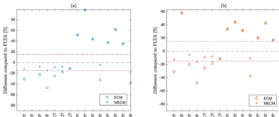
**Fig. 12.** Percentage deviation of ECM and MECM results to FLTA results for site 3 (a) and site 14 (b). The 50-years contour uses a 90% percentile, while the cut-off contour uses a 50% percentile.
