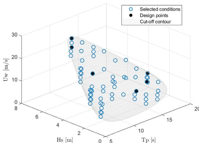
**Fig. 11.** Discretized conditions for cut-off contour surface for site 14. The blue circles are the selected conditions, while the filled black circles are the design points.
