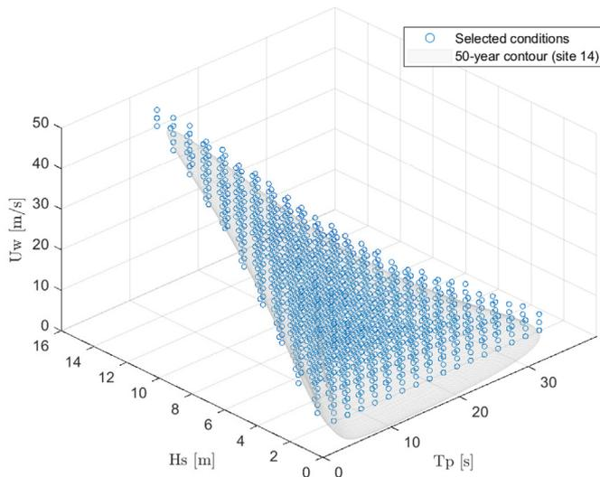
Fig. 5. Environmental conditions used for FLTA. The 50-year contour surface of site 14 is included to visualize the threshold of the selected conditions.
