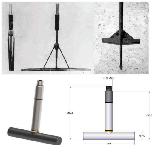
Figure 1. The Iskyrometer (top left), column penetration test (top right) and T-bar used in this study (bottom). The T-bar was \text{\O}40 mm and width 250 mm (tip area 10,000 \text{ mm}^2 ). The drilling rod is \text{\O}36 mm (area \sim 1,000 \text{ mm}^2 ). Sources: Kallstenius (1961), Massarsch (2014), Geotech (2019).
