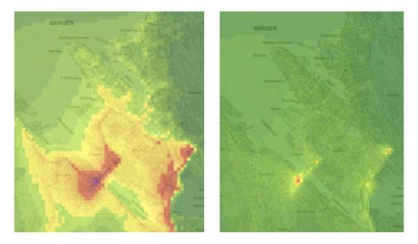
Figure 1.3: PM10 (left-hand side) and PM2.5 (right-hand side) concentration in Bergen city center (Miljødirektoratet, 2022).
