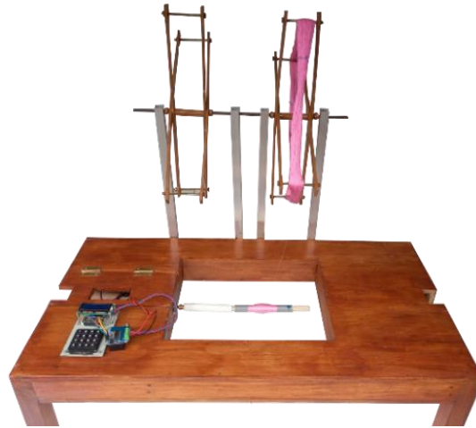
Figure 3: Mechanical Design of Automatic Thread Winding Tool.
