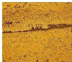
c) A crack in parent material
