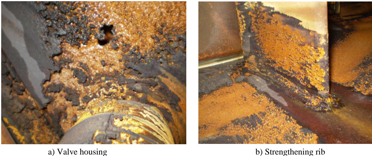
Figure 11. Damages detected at the synchronous valve
