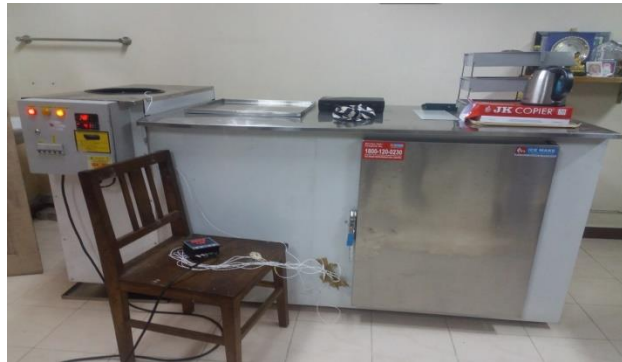
Fig. 3 Experimental set up of a heat pump dryer
