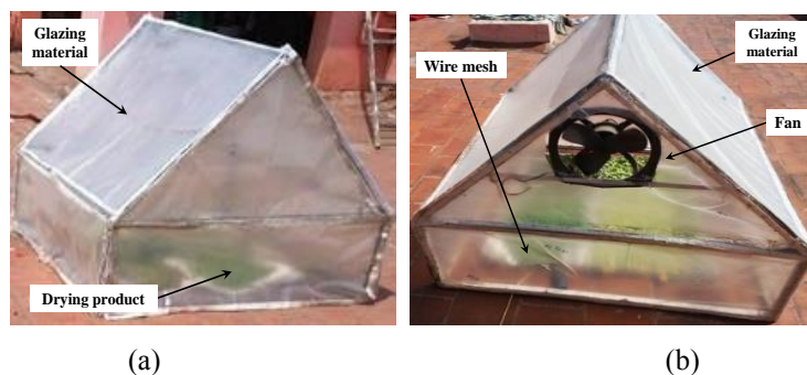
Fig. 2 Greenhouse dryers in (a) Passive mode (b) Active mode
