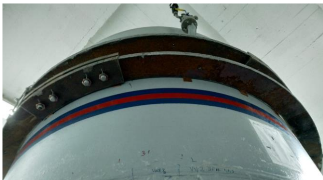
Figure 12. Stiffener bonding with 4 screws M30 (class 8.8).
